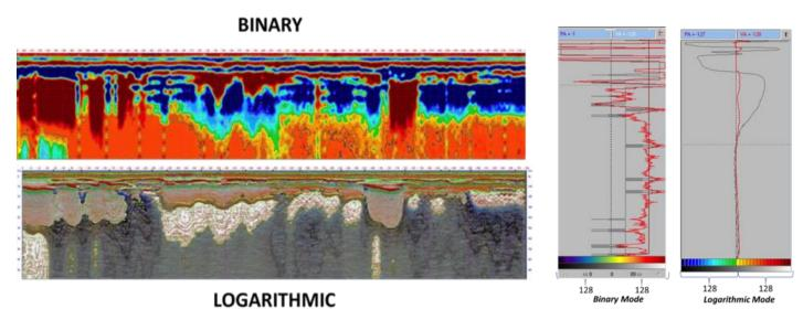
Fig 2: Recording of the EM wave, showing different parameters - binary is a "quick method" using just one pulse of energy, Logarithmic uses many pulses to determine more detail.
