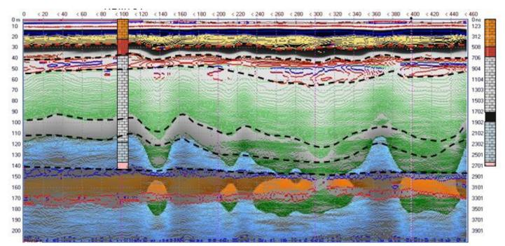
Fig 6. LF Radargram with borehole lithology overlaid.
