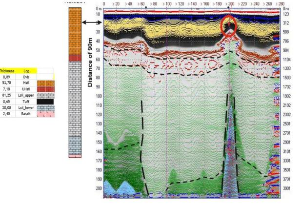
Fig 8. LF data with borehole correlation and showing a vertical karstic feature.
