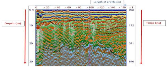
Fig 3. Radargram illustrating scales
