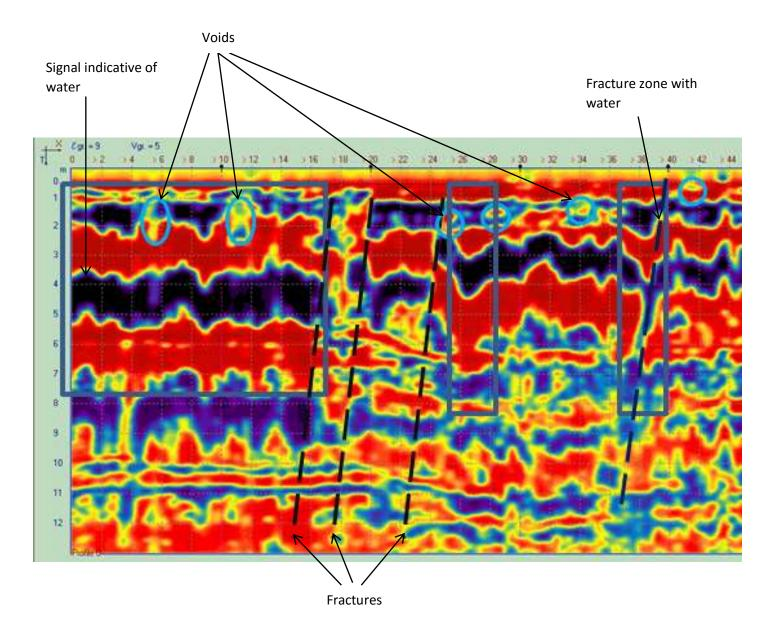
Fig 8. Radargram showing the fractures, voids and water zones interpreted from a section in the tunnel.
