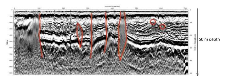
Old Mine Working/collapse/void
