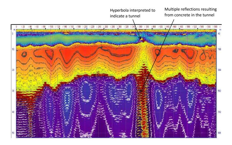
Fig 7. Radargram showing a void at 5 m depth interpreted as an old mine working.
