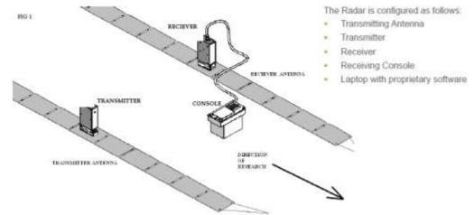
Fig 2. Antennas are more commonly moved one behind the other (series) however for diagrammatic purposes are shown here in parallel.
