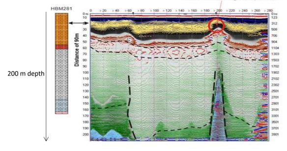
Fig. 10: Above Radargram shows Terravision data using REFLEX software to 50 m depth. The lower Radargram shows data from a different profile line in the Terravision software krot to 200 m depth
