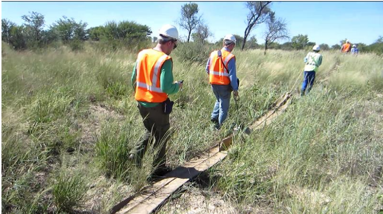
Fig 6. 6m antennas collecting in series in the bush
