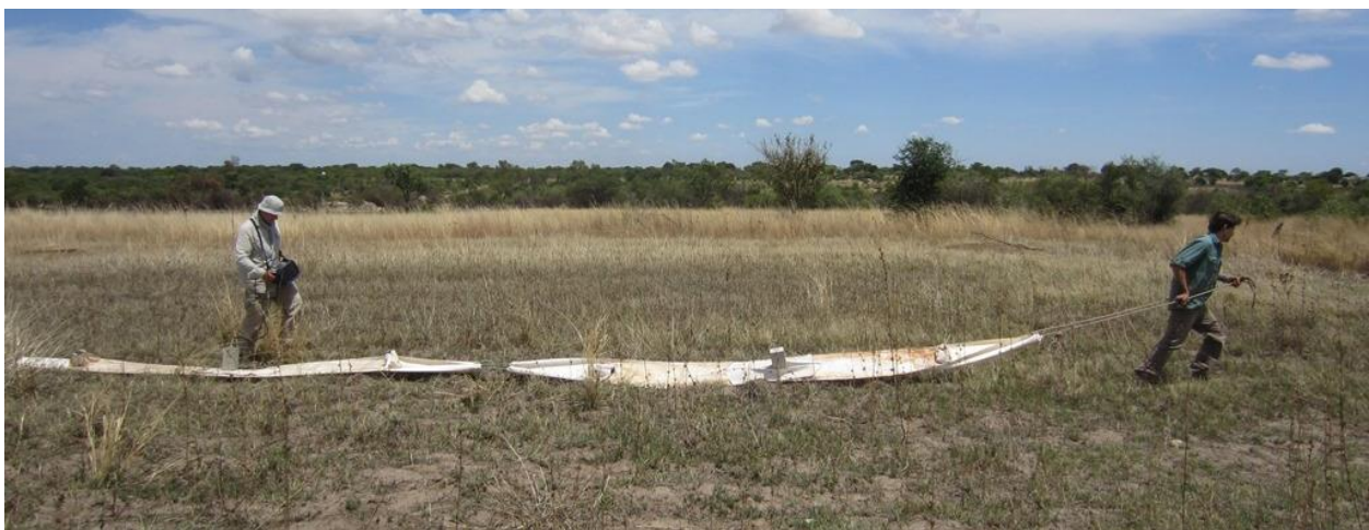
Fig 1. Terravision radar using 3m antennas and 10MW transmitter. Africa 2014
